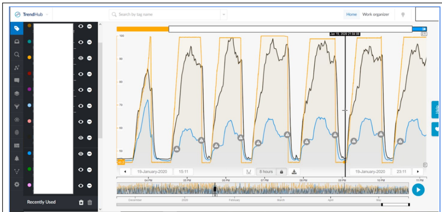
Figure 2 - Oxygen Concentration of a Biological Wastewater Treatment Plant Over Time. (Source: TrendMiner)
